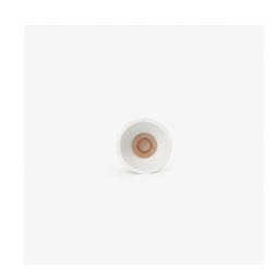
TULIPA is the ideal solution when light quality and great visual comfort are needed. It is a white downlight with aluminium injection frame and high - quality finishes which, thanks to its cut - off and its integrated honeycomb—which you can choose—, guarantees maximum visual comfort. This TULIPA recessed has a colour temperature of 2700K, an angle of15°, a power of 7W, CRI90 and with control system triac.
