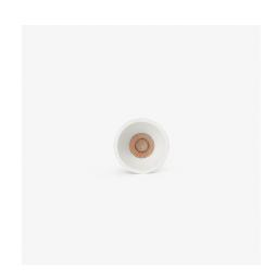
TULIPA is the ideal solution when light quality and great visual comfort are needed. It is a white downlight with aluminium injection frame and high - quality finishes which, thanks to its cut - off and its integrated honeycomb—which you can choose—, guarantees maximum visual comfort. This TULIPA recessed has a colour temperature of 2700K, an angle of24°, a power of 7W and CRI90.
